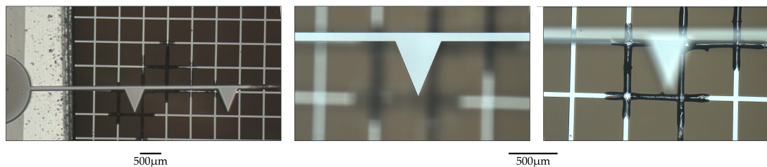
Figure 11. A typical failure mode of an electrode set. Permanent damage is sometimes observed following sparkover from a wire tip to the collector grid. This may be due to the relatively high current density following dielectric breakdown causing rapid Joule heating in the grid wires, or due to physical ablation during the high current breakdown. After a destructive event such as this, both electrodes were replaced despite there being no visible damage to the emitter wire.
